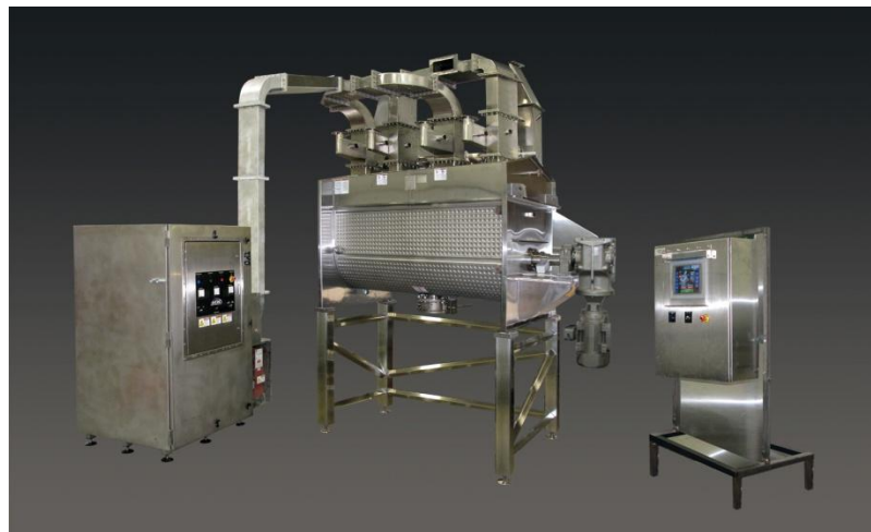
Microwave mixer designed to dry a proprietary chemical compound
