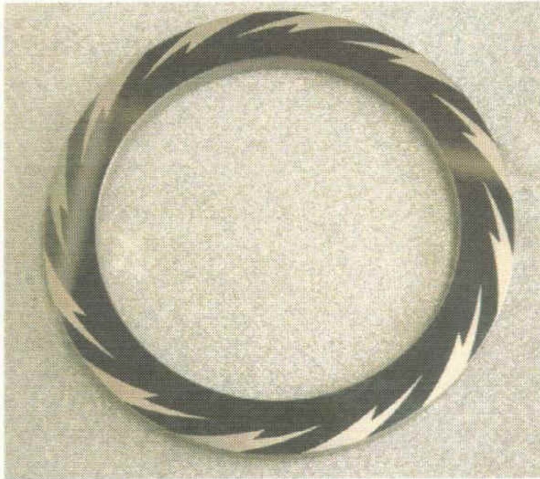
Figure 4 - Grooves in Seal Mating Ring
