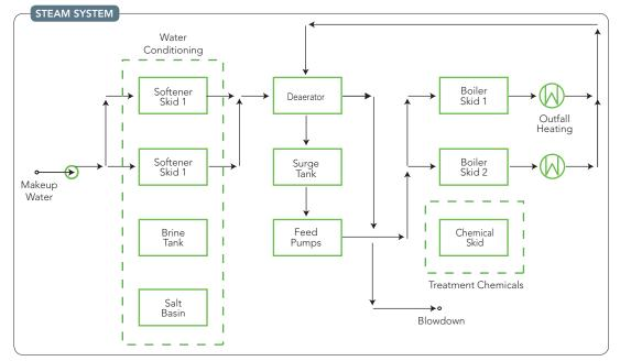
Figure 1. The relatively complex flow scheme sprawls over 14 P&IDs.
