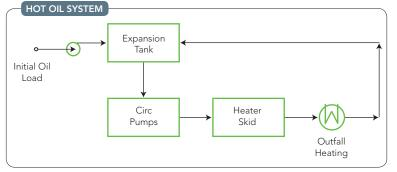
Figure 2. This simpler and cheaper option requires only four P&IDs.
