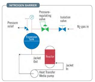
Figure 1. Nitrogen blanketing not only creates a barrier between the heated fluid in the expansion tank and the outside air, but also helps prevent the fluid's vapors from escaping into the atmosphere.
