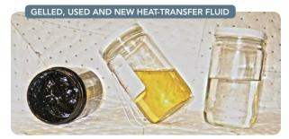
Figure 2. If a cooled sample won't pour, don't shut down your system until you have a plan to remove and replace the fluid.
