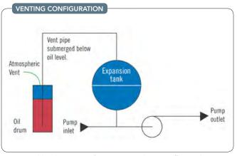
Figure 2. Cold-seal venting configurations provide a cost-effective alternative to nitrogen blanketing when vapors from the heat-transfer medium are not hazardous or undesirable.
