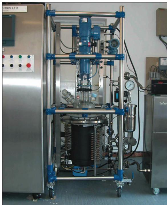
Figure 2. This “constant flux” reaction calorimeter recently got its first plant use at Clariant Chemicals' Leeds, U.K., site. Source: Ashe Morris
