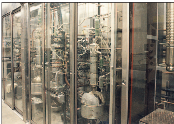
Figure 3. Large, heavily automated group of distillation pilot plants provides major savings in design and construction as well as more efficient operation.
