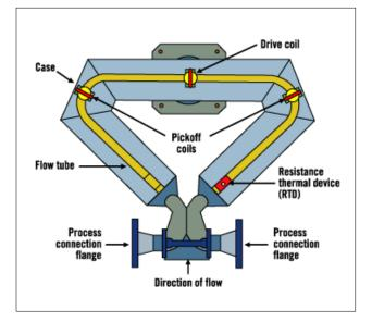
Figure 2. Coriolis meters offer volumetric flow, fluid temperature and density, and calculated density-type variables. Drawing courtesy of Micro Motion
