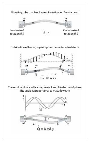
Figure 3. The Coriolis effect is generated, as it is in the double curved tube, through the rotation of the tube about fixed ends. The two sine waves on the inlet and the outlet are shown as Point A and Point B. The inlet side lags the outlet side, which is identical for either straight or curved tubes.
