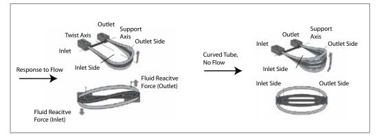
Figure 1.In a dual-tube Coriolis meter, the two vibrating tubes rotate around the fixed end points. When fluid is flowing, reactive force on the inlet side is opposed to the motion of the tube, twisting it ever so slightly. The amount of twist is proportional to the mass flow rate.
