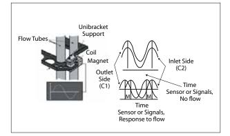
Figure 2. To exploit the Coriolis phenomenon, a magnet is attached to one tube and a pickoff coil is attached to the other tube at the inlet and the outlet. Under flow conditions as the tubes twist, the generated sine waves shift apart. The instrument measures the twisting, which is directly proportional to the mass flow.
