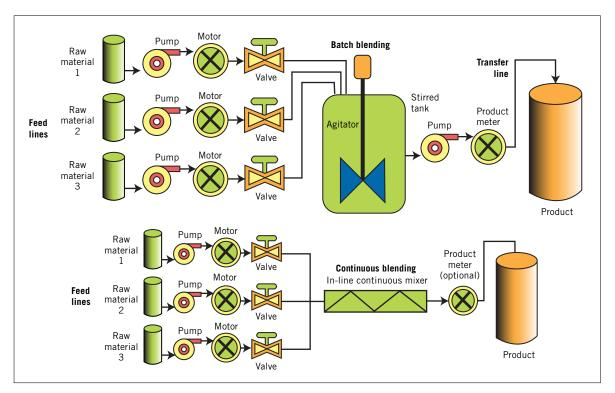
Figure 1. Continuous blending requires smaller equipment, less floor space and a smaller product storage area than batch blending.
