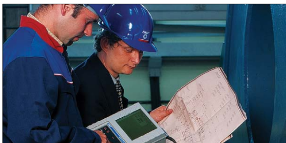
Figure 2. Portable unit stores and analyzes data which also can be uploaded to a computer for more detailed analysis.
