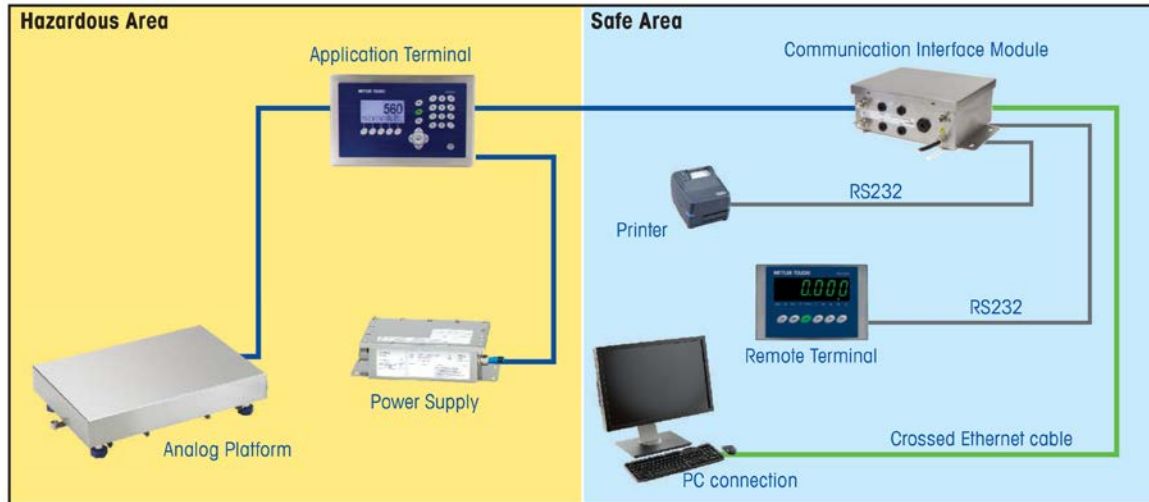
Figure 4. An analog weighing platform and intrinsically safe weighing terminal communicate to standard peripheral instruments, such as PC, through a special barrier.
